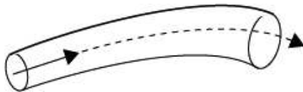
Figure 1.1 A portion of a vortex filament. The product of the vorticity (indicated by the arrows) by the normal section of the filament is a constant along the filament. It is also invariable during the motion of the fluid.
